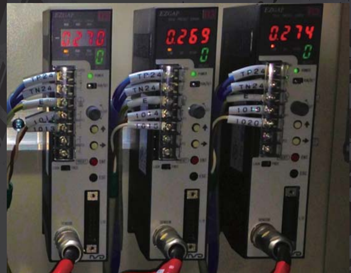
Actual EZ GAP (NSD's eddy current displacement sensor for rubber thickness measurement) converter which is installed at calendering machine.
